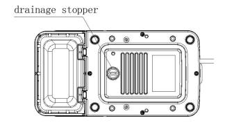
Note: If found water leakage from the bottom, pls tighten the drainage stopper.
